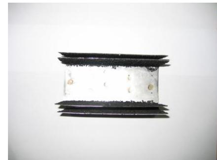
Small size Activated carbon coated Cryopanel
