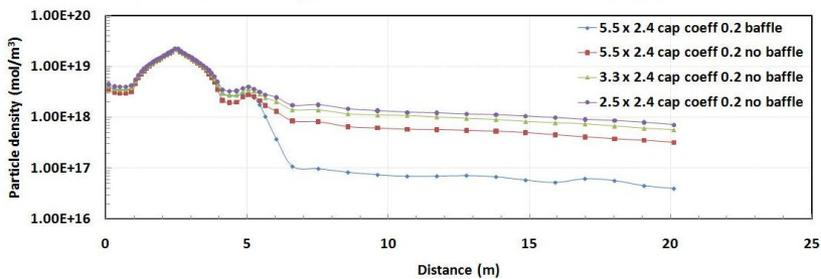
comparison of particle density profiles with and without baffle and different pump dimensions
