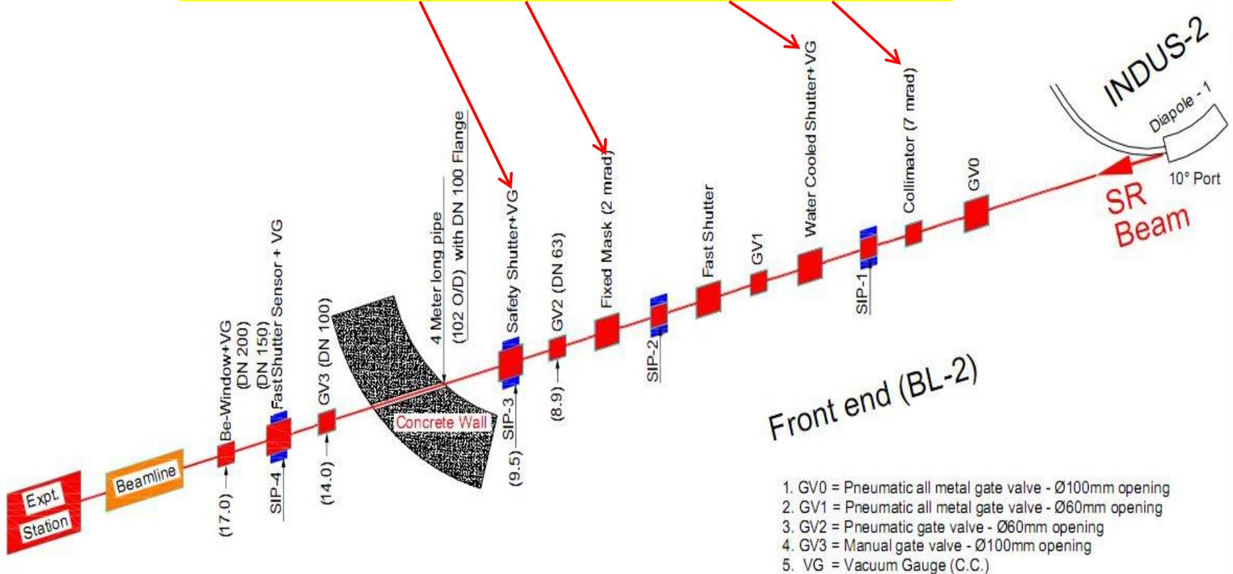
1. GV0 = Pneumatic all metal gate valve - Ø100mm opening
