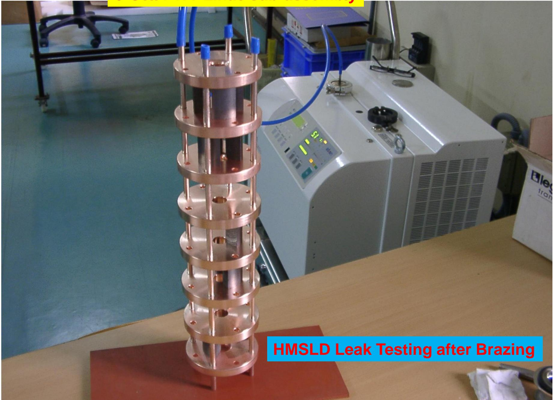
HMSLD Leak Testing after Brazing
