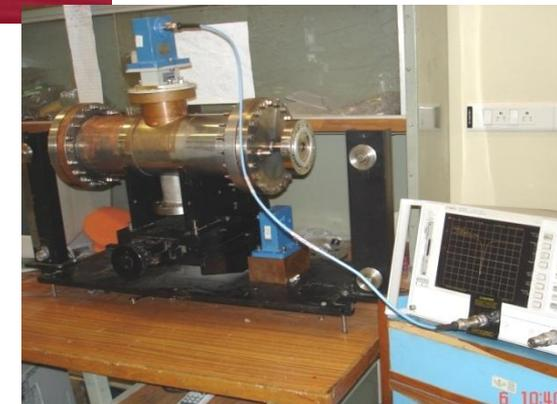
8 Cell PWT on low power RF test stand
