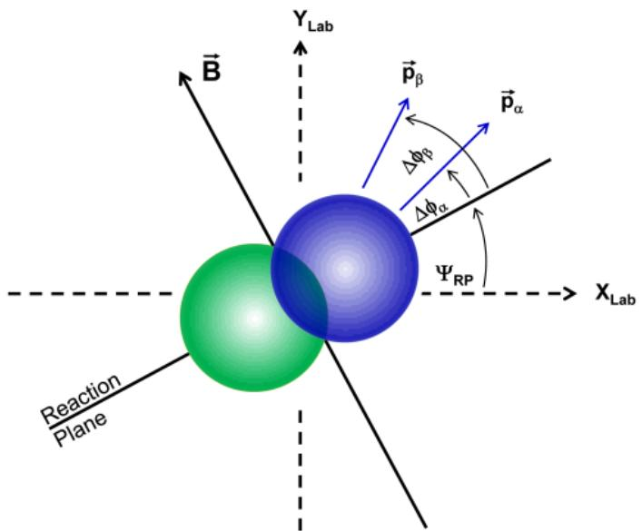
$$\gamma^{ab} = \langle \cos(\phi^a + \phi^b - 2\psi_{RP}) \rangle. \quad (1)$$
