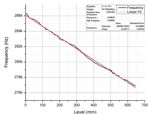
Figure 4: Output frequency vs level along with a linear curve fit
