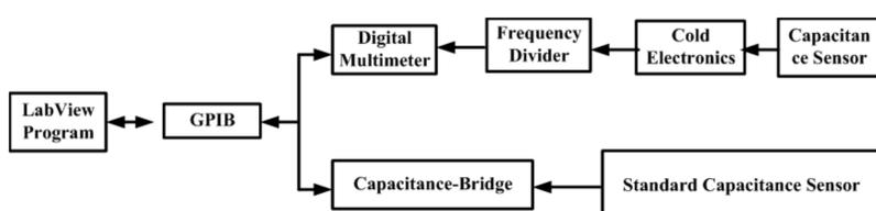
Figure 2: Schematic of interfacing DAQ
