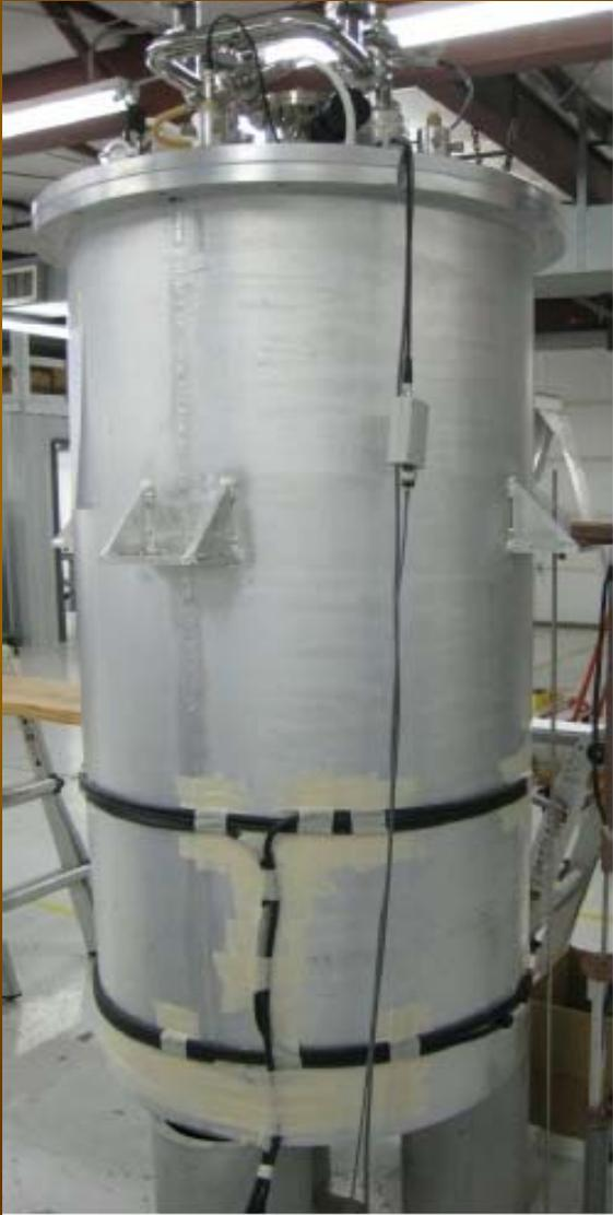
A persistent mode superconducting magnet with shim coil assembly
